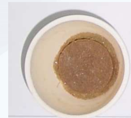
Digestion with \text{CaSO}_4 / \text{CaCO}_3 (950 °C)
