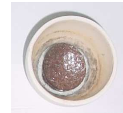
Digestion with \text{Na}_2\text{SO}_4 (1050 °C) → partial melting!
